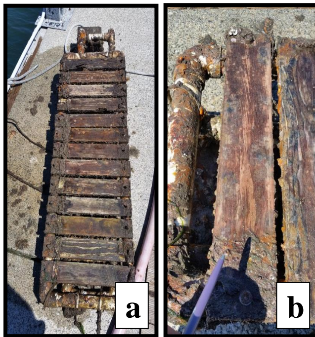
Figure 2.5: Example of a (a) Marine borer test racks. (b) and a western juniper sample attacked by marine borers (6-month exposure).
