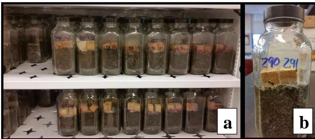
Figure 2.6: Soil Block Test. (a) Soil block jars in incubator. (b) Soil block jar after 16-week incubation period
